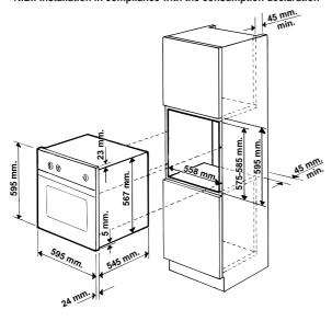
that it rests on two strips of wood is preferable. If the oven rests on a continuous, flat surface, there must be an aperture of at least  $45 \times 560$  mm.
